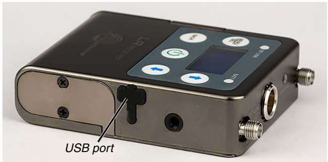
Top panel provides antenna ports, IR interface and balanced audio output. The belt clip also attaches the shoe mount adapter.
